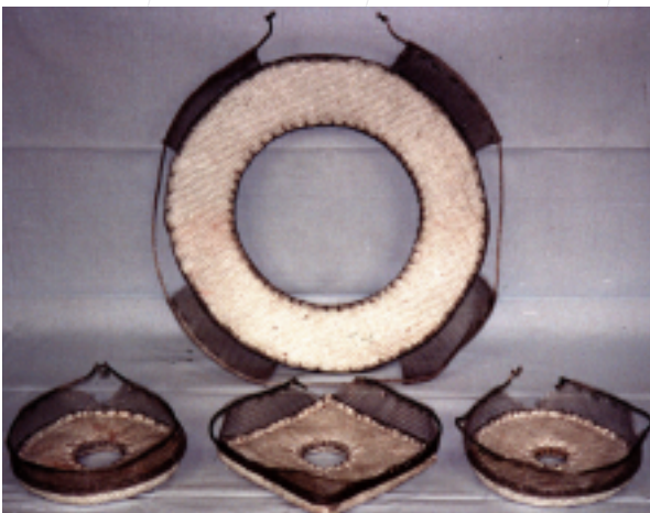
Burner and Draft Probe Gaskets in the forefront with Exhaust Manifold Leg Seal Gasket stood on edge in the background.
